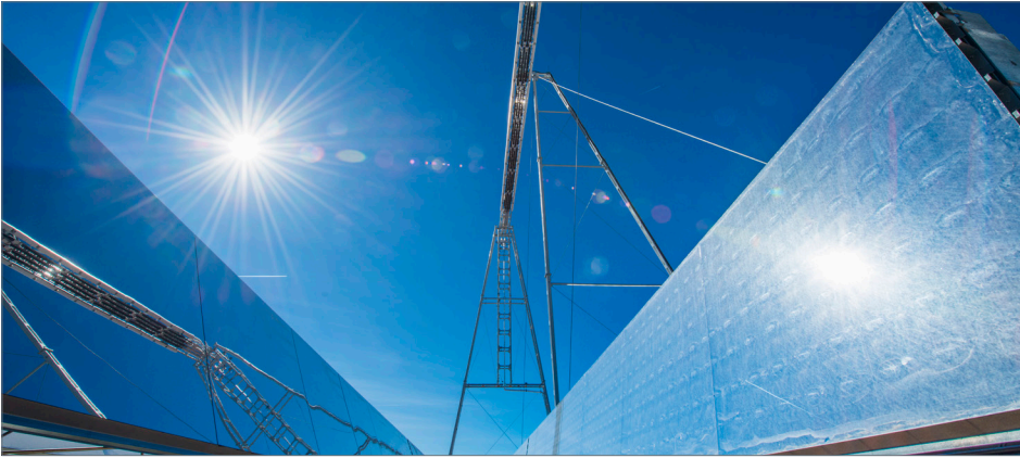
The molten salt test loop (MSTL) at Sandia National Laboratories' National Solar Thermal Test Facility in Albuquerque, New Mexico. AREVA's solar team and Sandia's molten salt technology experts have developed an innovative approach to energy storage that combines the MSTL with AREVA's Compact Linear Fresnel Reflector applications. (Photo by Randy Montoya, Sandia Labs)
