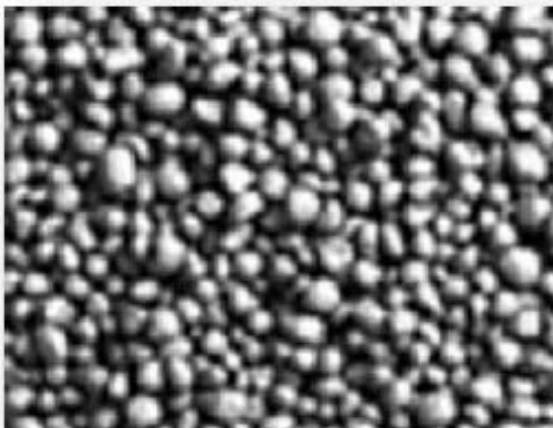
Typical ceramic proppant 20/40
