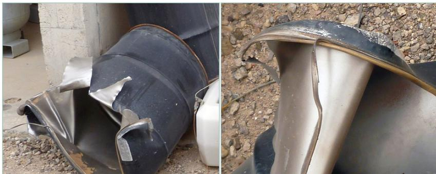
**Figure 1-1. Views of exploded drum. The left image and the close-up image on the cover show the bottom of the exploded drum. The right image is a close-up view of the bottom seam of the drum.**
