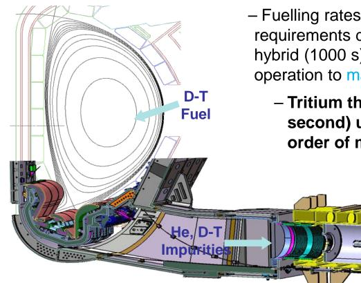
Fuelling rates and Torus pumping requirements differ for inductive (450 s), for hybrid (1000 s) or for steady state (3000 s) operation to maintain the plasma operation
