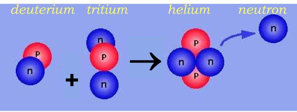
• The energy released from 1 gram of fused DT equals the energy from about 2400 gallons of oil
