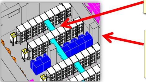
First confinement system Inert glovebox and its extensions
