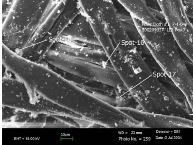
SEM images of lint free cloth used to collect particles. Particle sizes ½ to 10-20 microns.
