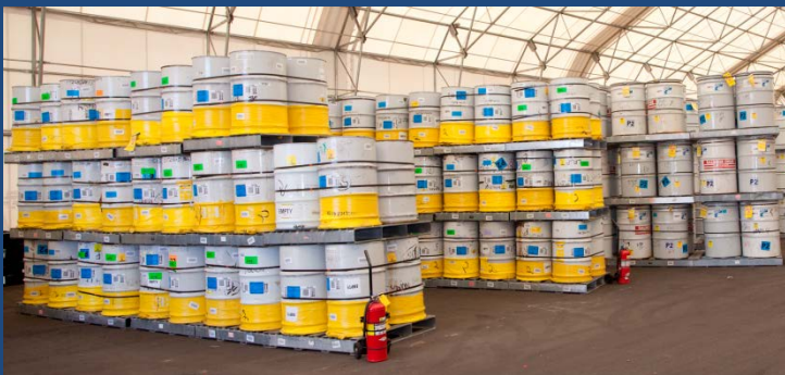
The waste stored above ground at Area G is in metal containers or under a fire suppression system on asphalt or concrete pads.
