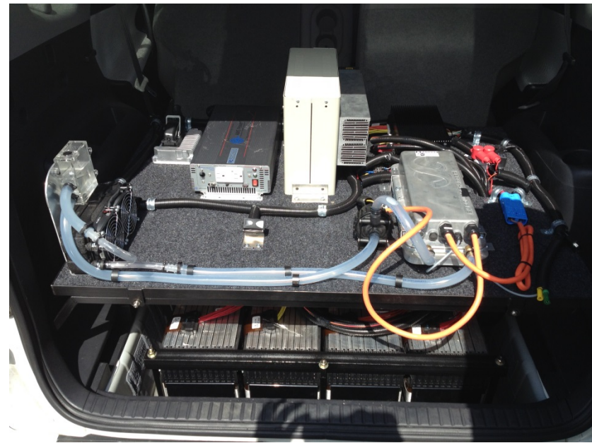
• Other electronics added by Toyota to have external charge & discharge path for the add-on battery pack (for integrity and as a back-up to wireless)
