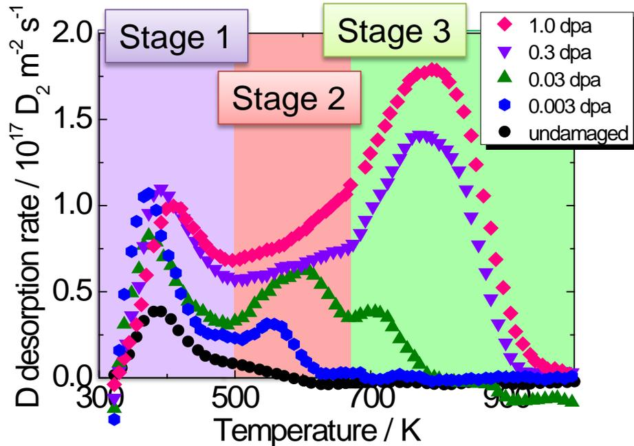
D<sub>2</sub> TDS spectra for Fe<sup>2+</sup> irradiated W with various ion fluence.
