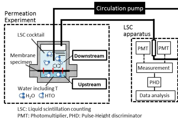
Successful observation of tritium permeation induced by water corrosion of pure iron
