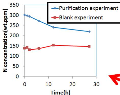
In the experiment, purification by pure Ti was confirmed in 27 hours.
