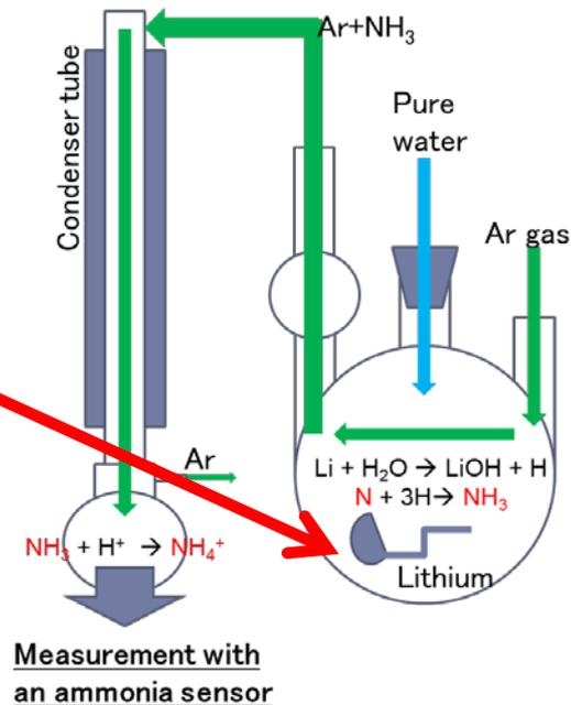
Measurement of ammonia concentration gives the nitrogen concentration in lithium indirectly.
