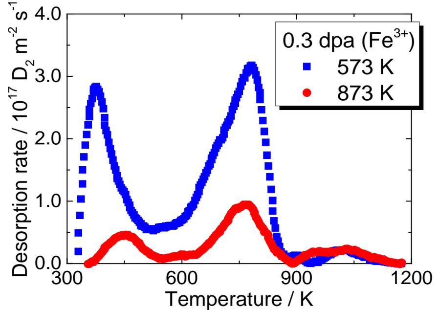
D<sub>2</sub> TDS spectra for Fe<sup>3+</sup> implanted W
