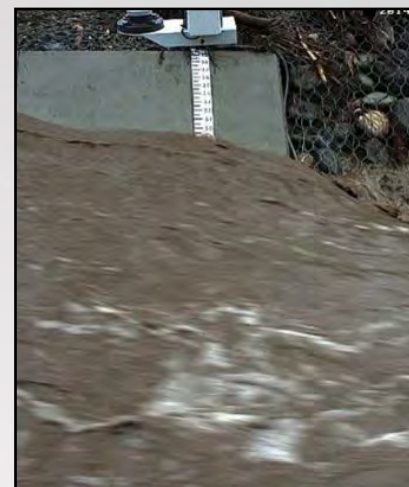
The E050.1 gage station in Los Alamos Canyon measures storm water flowing at 7 p.m. (left) and one hour later at 8 p.m. (right).
