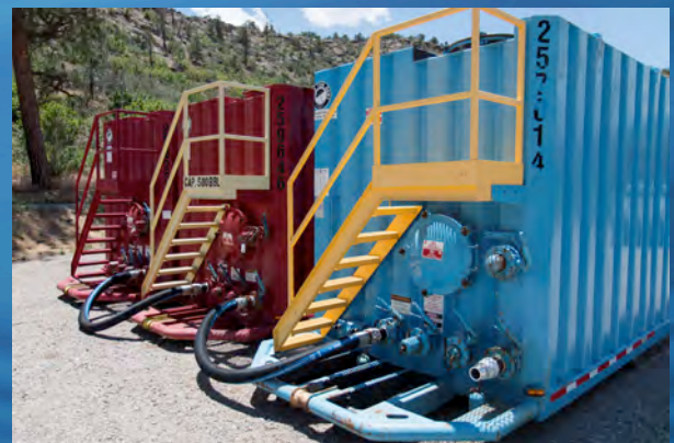
Portable storage containers are used at the site to hold water.
