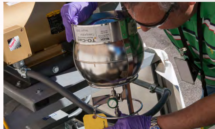
Crews conduct periodic sampling at both units using SUMMA canisters. After the samples are analyzed, technical experts use the data to determine concentrations of VOCs and mass of VOCs removed.
