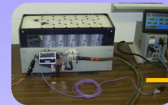
Li-ion battery and BMS
