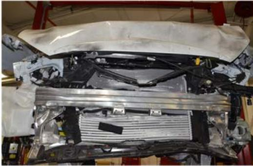
Extruded Aluminum Front Bumper and Crush Can
