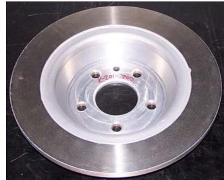
(a) Coated Rotor Prior to Test
