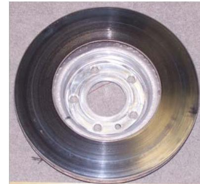
(b) Coated Rotor After Test
