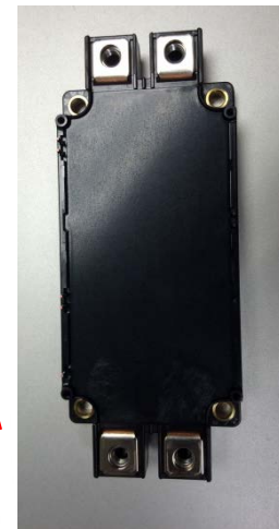
1200 V, 300 A SiC MOSFET commercial single phase module
