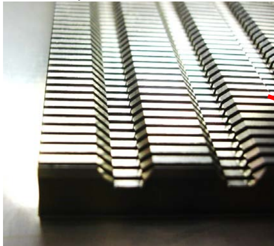
Close-up of fins on bottom of power module
