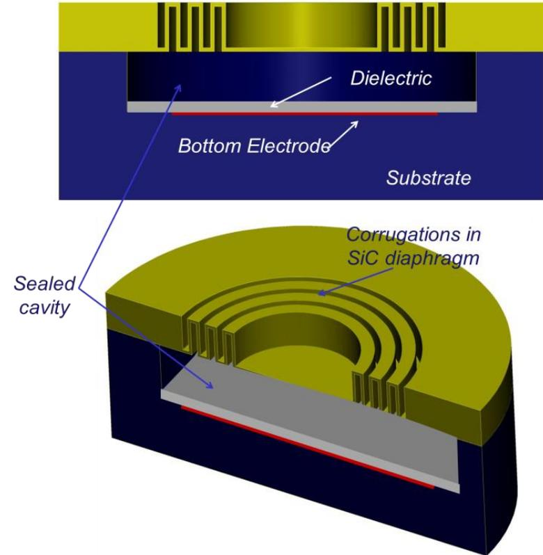
*Schematic images of proposed design for capacitive pressure sensor
