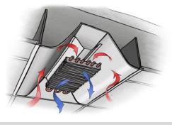
Figure 1: Passive Chilled Beam Design
