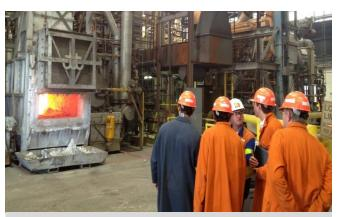
University of Dayton and University of Kentucky IAC students evaluate the operation of a large reverb aluminum melt furnace located at a smelting facility in Kentucky.
