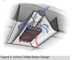
Chilled beams are more efficient than conventional VAV building systems because of the heat storing capacities of air and water. One cubic foot of air at standard temperature and pressure has a heat capacity of 37 J/K, while water has a heat capacity of 20,050 J/K.
