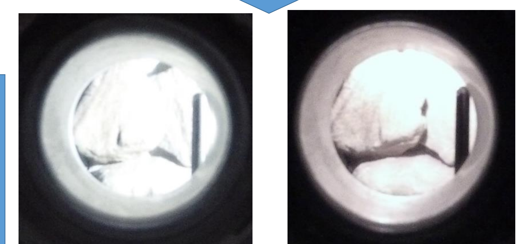
Figure 6, 250°C Oven Lighting Test: (Left) SiC LEDs, 0.02A:3V; (Right) Oven Bulb 1A@7V
