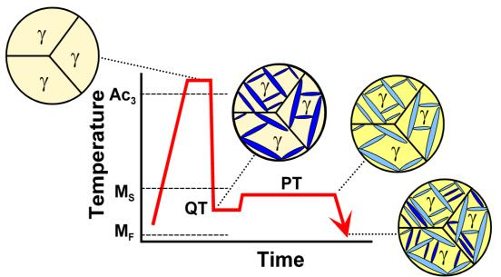
• Alloying, processing, microstructural evolution and mechanical properties inter-relationships are being studied.
