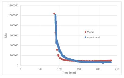
The first comparison of the LSU gPROMS computational modeling and Tulane ACOMP experiment are shown for free radical polymerization of MMA in butyl acetate, initiated by AIBN. Early results are promising
