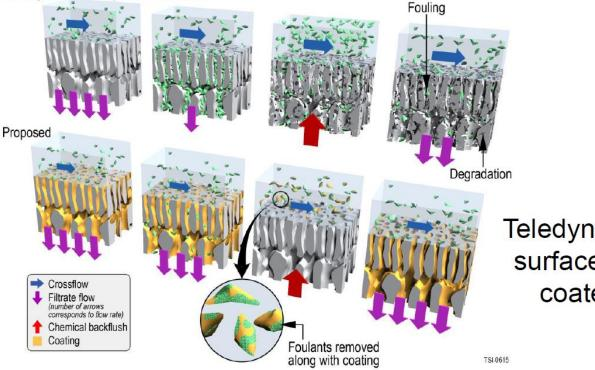
Teledyne coating: both membrane surface and inner pore walls are coated without affecting flux
