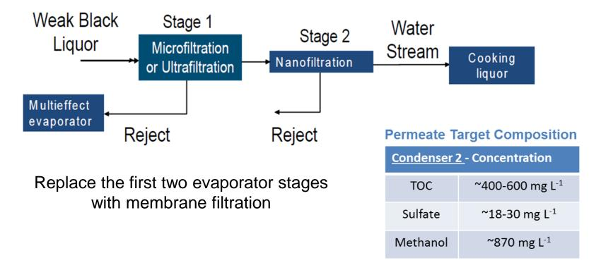
Alternate processes such as coagulation, ion exchange can be added to ensure all target product quality specifications are met when preparing cooking liquor. We will not add additional salts to ensure salt concentrations do not increase over time in this closed loop system.
