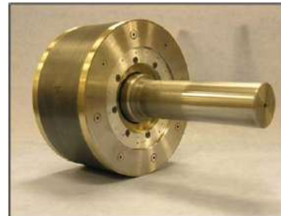
Prototype permanent magnet motor with brushless field excitation coil operates at 16,000 RPM
