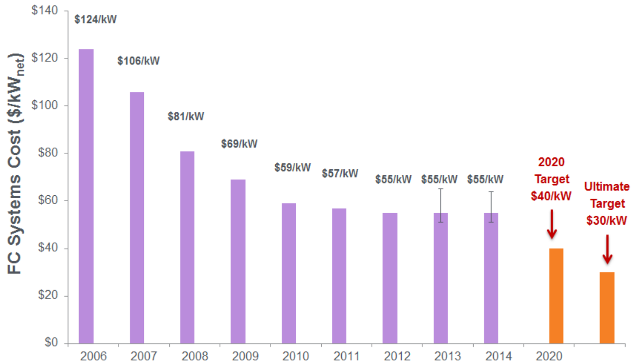
Figure 1. Modeled cost of an 80-kW net PEM fuel cell system based on projection to high-volume manufacturing (500,000 units/year). Reported values from 2012 and earlier were adjusted to account for the higher platinum price, the realigned compressor and expander efficiencies, and the Q/ΔT requirement introduced in 2013 (see 2013 cost record).
