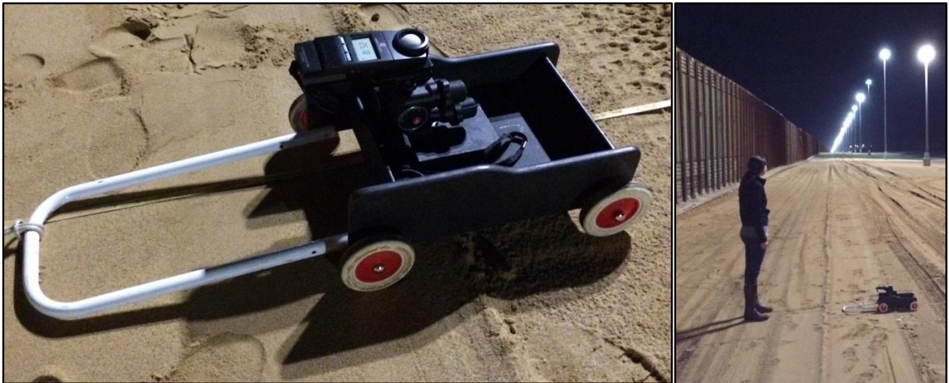
Figure 6. Illuminance Measurement Wagon. The illuminance meter was mounted on a tripod head, and the tripod head was attached to the base of the wagon. The knobs of the tripod head were used to adjust the front and lateral tilt of the illuminance meter to level the meter—with reference to the tripod head's leveling bubble.
