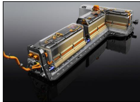
Chevy Volt Exceeding 50,000 Vehicles 16.5 kWh per pack ~825MWh
