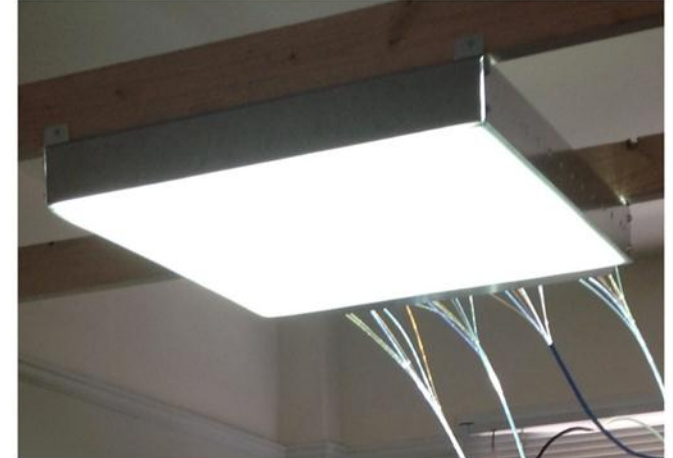
2'x2' Daylight Fixture
