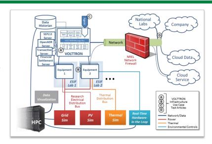
**Key Issues**: NREL is leveraging the VOLTTRON platform to extend the ESIF testbed to facilitate transactional interaction of equipment, the grid, and software components.
