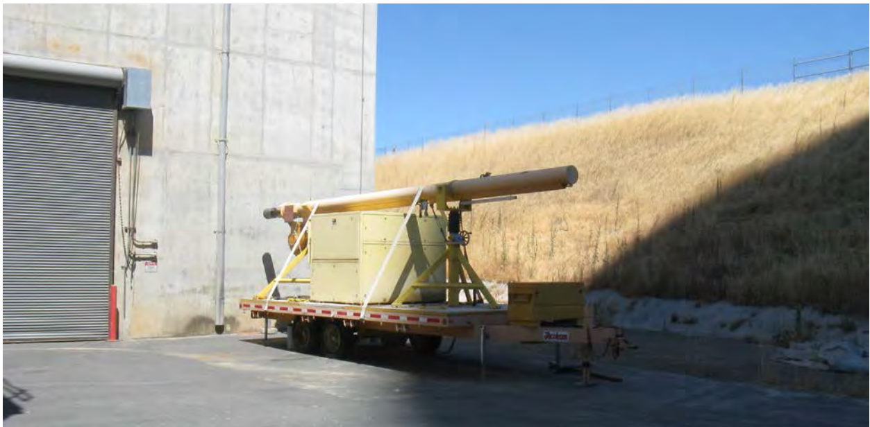
Figure 2-81. Hydraulic Ram Used to Emplace and Withdraw Canisters from Horizontal Storage Modules at Rancho Seco
