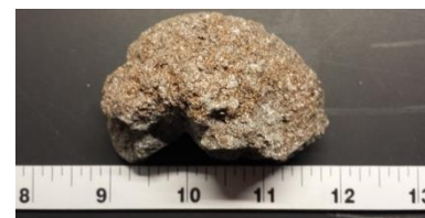
Agglomerated bed material after feeding corn stover
