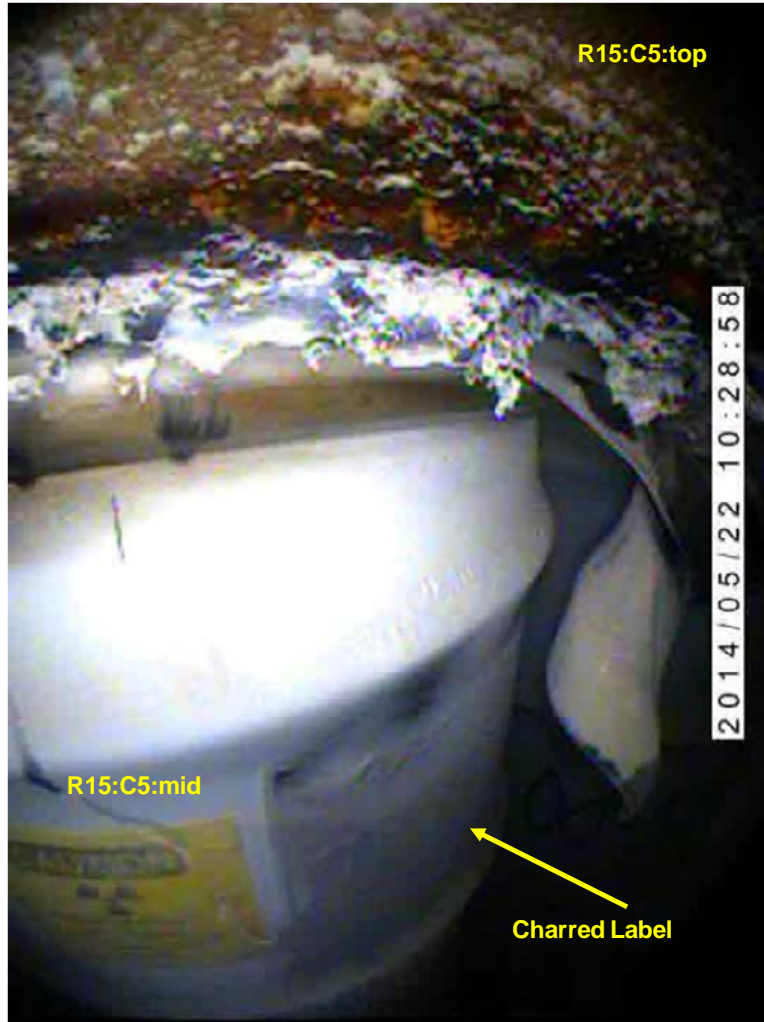
Figure 6-39: Charred Label at R15:C5
