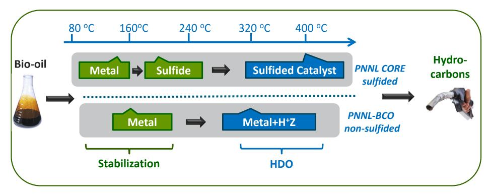
Reduced metal catalysts are required for low temperature stabilization of bio-oil by hydrogenation to eliminate gunk/coke formation and enable long-term operation.
