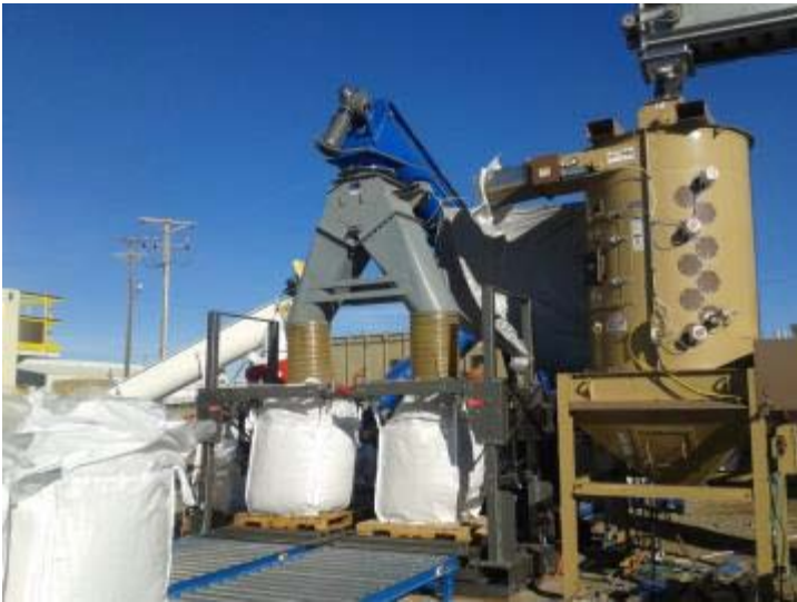
Transferring to the supersacks
