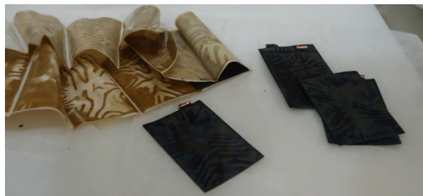
Figure IV - 58: Photograph of the anode and separator material from cell B
