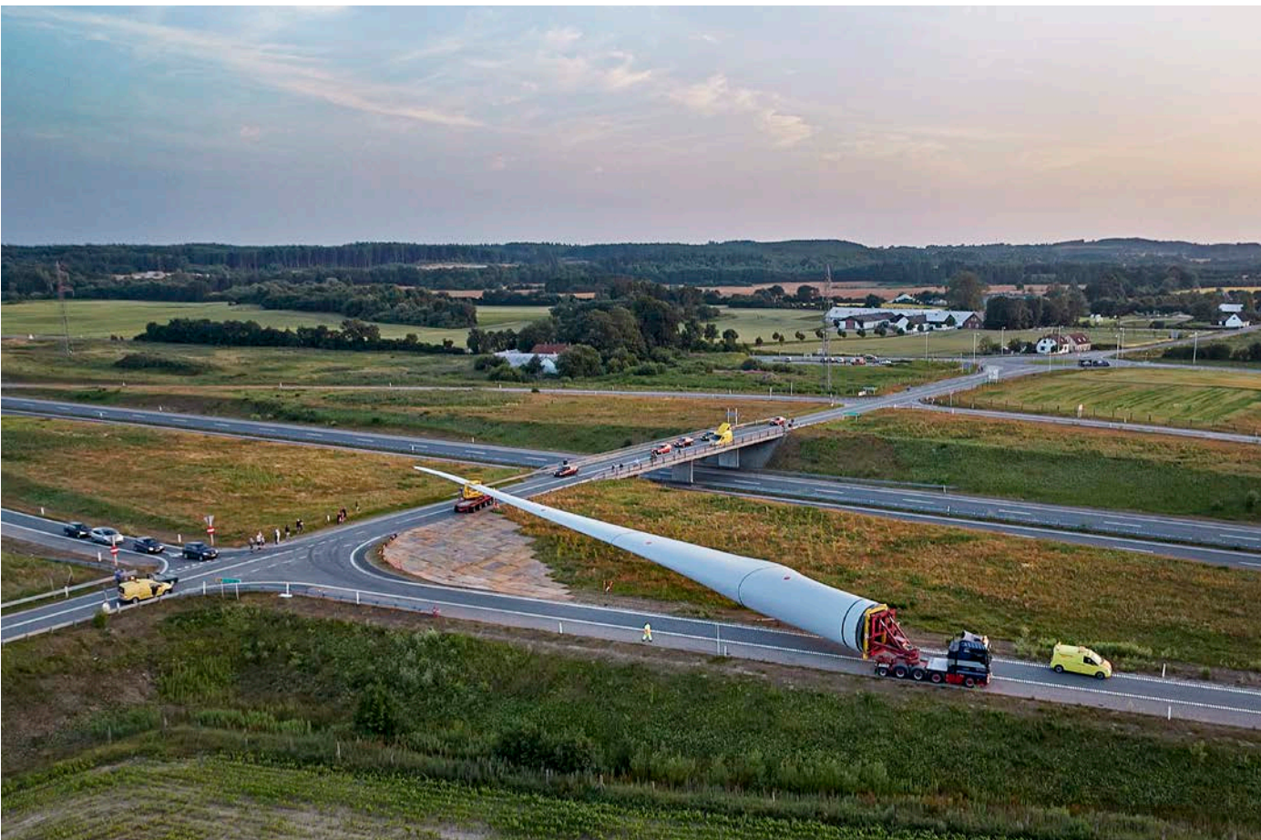
Figure 2-38. Example of wind turbine blades transportation obstacles
