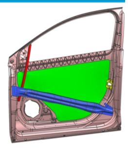
The magnesium door inner produced during this project (right) will be cast to shape, compared to an equivalent steel stamped door inner (left), which is made of multiple pieces that must be welded, thus requiring additional manufacturing steps. *Graphic image courtesy of General Motors*.
