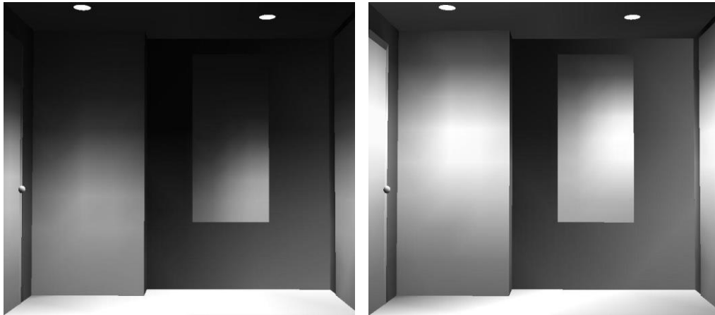
Entry area rendering comparing PAR halogen (left) to LED (right). LED increased vertical illuminance by 50%.
