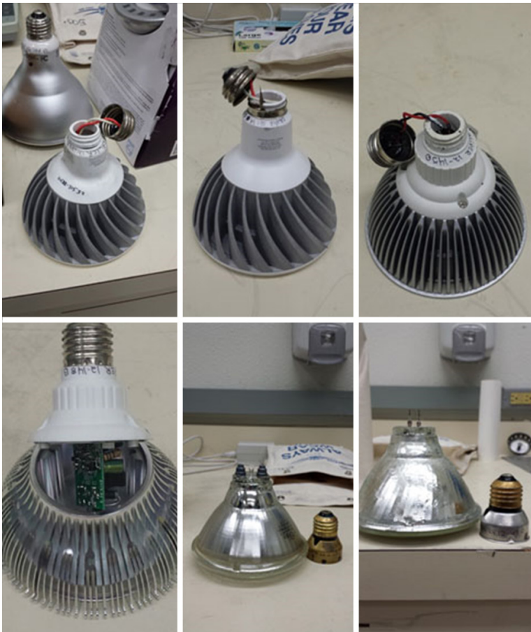
Figure 7. Examples of products experiencing physical damage that prevented further testing and therefore constituted catastrophic failure.
