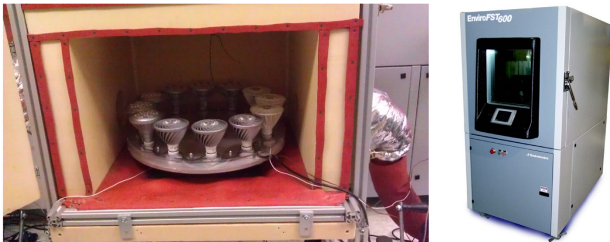
Figure 1. LEFT: Mechanical stress chamber housing 12 lamps. RIGHT: Environmental chamber that provided the thermal stresses.
