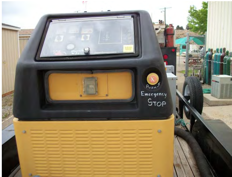
Figure 5. Emergency Stop Button
