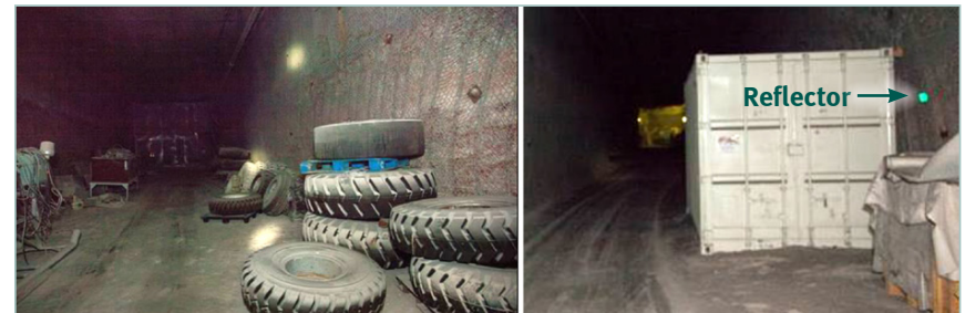
Figure 1-6. Combustible loading in the drifts and an obscured reflector
