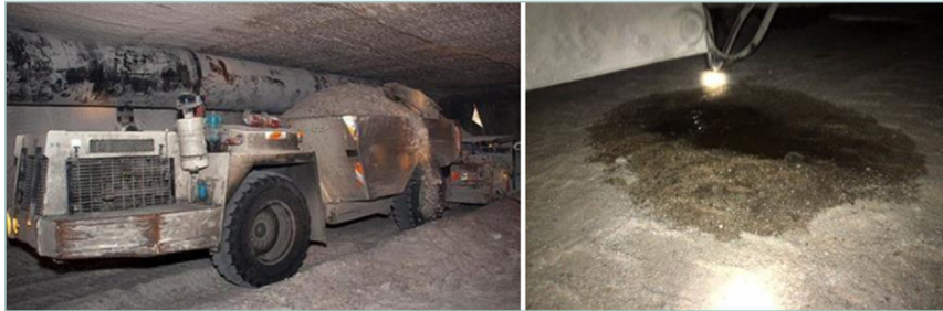
Figure 1-5. EIMCO Haul Truck 74-U-006A (similar to burned truck) and hydraulic fluid leak
