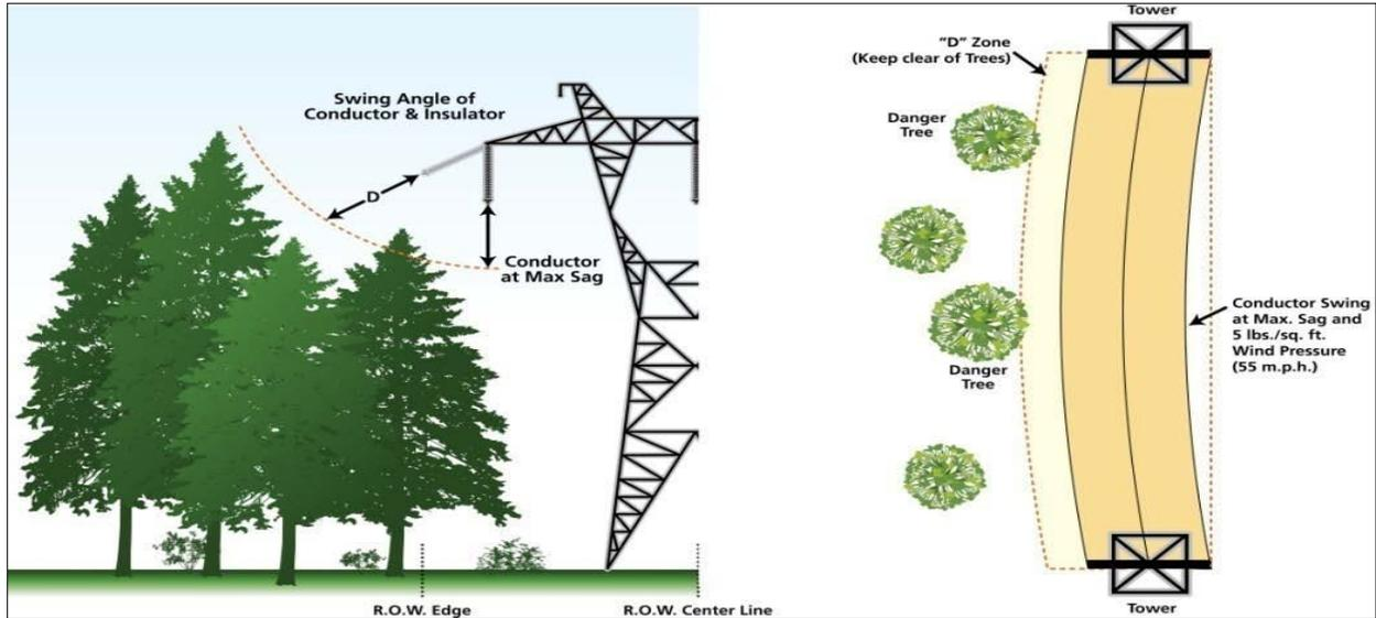
Fall-in trees (Figure 2-7) are any trees that, if they were to fall toward the transmission line, would extend into the minimum clearance distance to the conductor.
