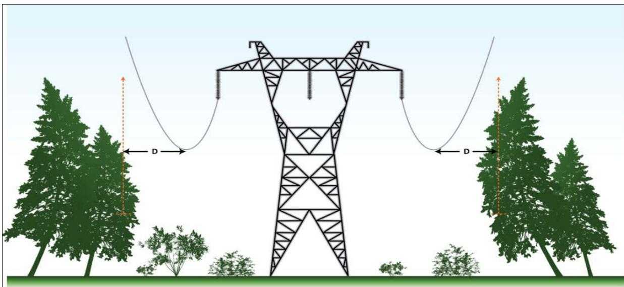
Grow-in trees (Figure 2-5) are located within and/or adjacent to the right-of-way; they have grown, or will grow, horizontally and vertically into the minimum clearance distance to the conductor
