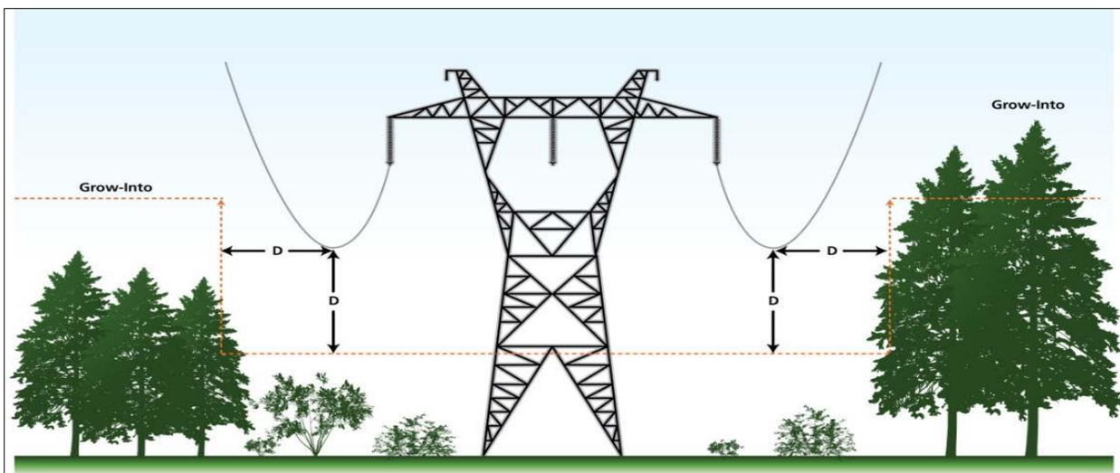
Swing-in trees (Figure 2-6) are located off and adjacent to the right-of-way; their branches would, or could, violate the minimum clearance distance to the conductor because of the conductor being blown toward the tree.
