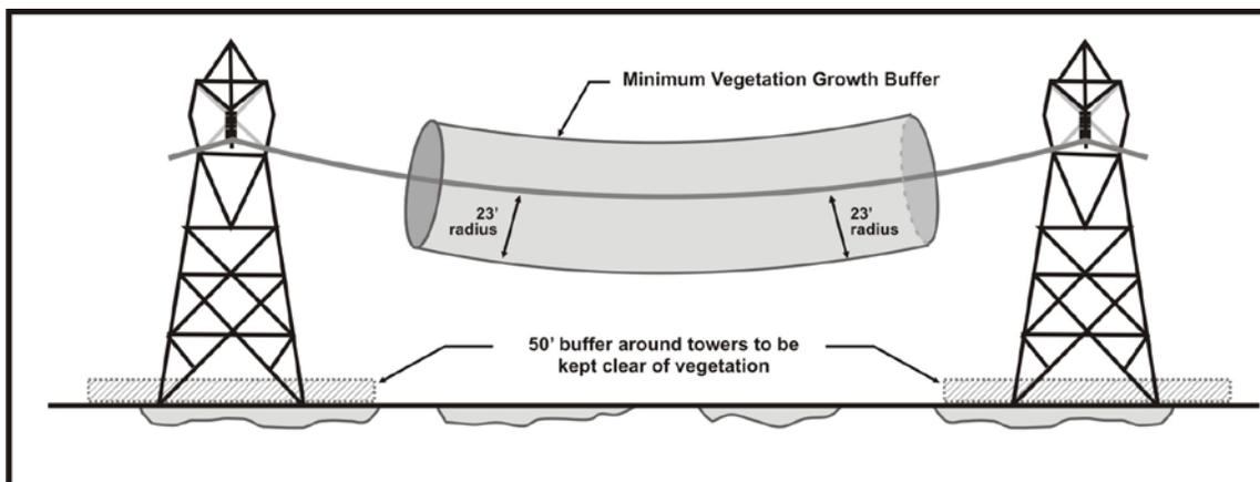
Bend-in trees (Figure 2-4) are located along the right-of-way; they have tops or branches that bend down or could bend down into the minimum clearance distance to the transmission line conductor.
