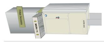
The filter box must be correctly sized for the appropriate filter, according to ACCA Manual D, taking into account pressure drop across the system. (Figure source: DOE 2014b)
