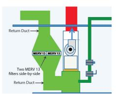
To increase surface area and reduce pressure drop for high-MERV filters, the return duct can be constructed to permit the installation of two furnace filters side by side, or deeper pleated filters can be used (Figure source: DOE 2014b.)
