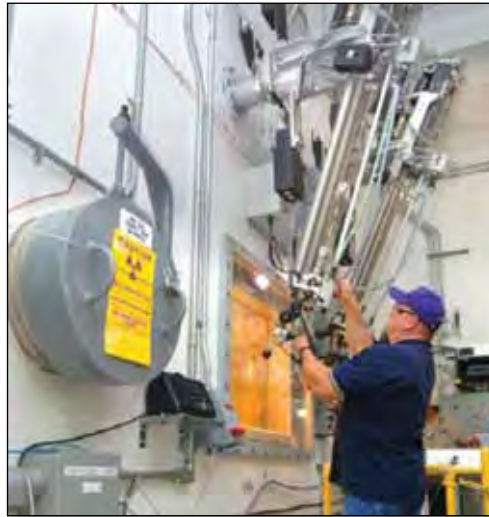
A worker manipulates RH waste at the TWPC.
