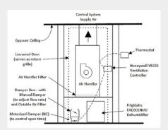
The two Broadmoor Development Corporation houses also installed supplemental dehumidification; however, these standalone dehumidifiers are located in the open return of the HVAC system, which is in a mechanical closet. The image above shows the schematic design and the photo below shows the dehumidifier installed in the open return with the outside air duct and filter/damper box on the left-hand side.
