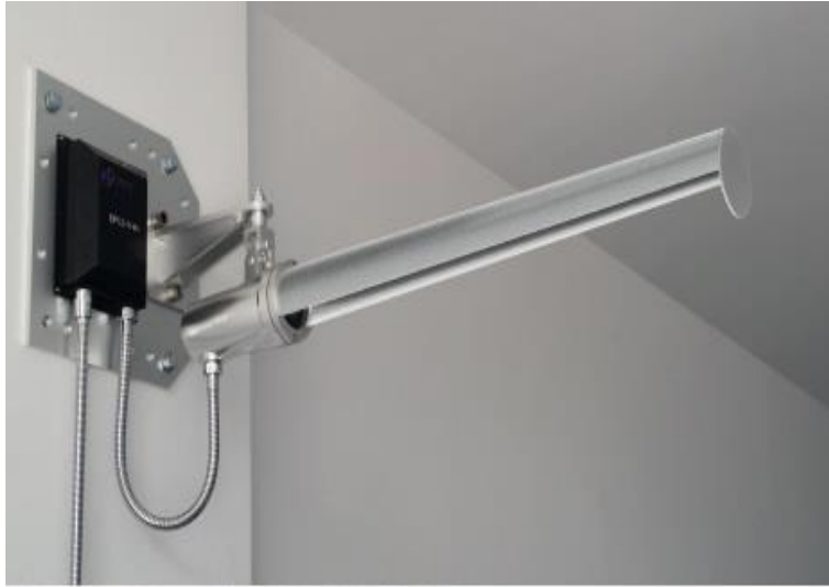
Open Path Reflection Laser Methane Detection System Powered by Solar Panels
