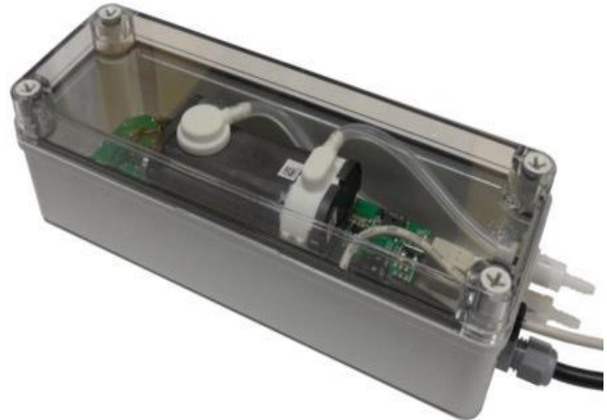
Integrated continuous sampling system for low parts-per-million (PPM) methane and hydrocarbon detection
