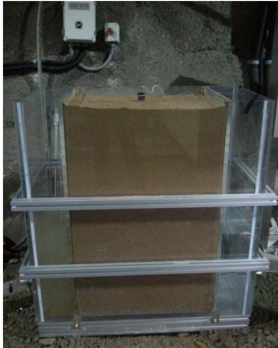
Figure 6-25. Sand box for SP sand box experiments (from Wang et al., 2014)
