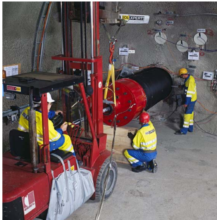
Figure 3-28. HG-A Experiment at Mont Terri URL: Installation of packer system (from Marschall et al., 2012)
