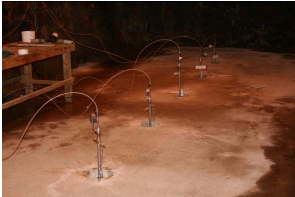
Figure 3-44. BRIE Experiment at Äspö HRL: The test niche and five boreholes (distance 1.5 m) used for initial characterization and selection of BRIE site (from SKB, 2011b)
