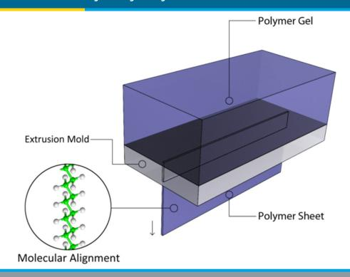
Illustration of continuous processing of UHMW-PE sheets (or fibers) with highly aligned molecule chains. UHMW-PE nanofibers are extruded through a template to form a continuous sheet (or fiber) and are stretched (not shown) further to align the molecules. *Graphic courtesy of MIT.*
