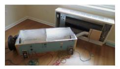
To test the airflow through the PTAC fresh air kit, the team used a custom device that combines a powered capture hood and an orifice plate. The pressure on the PTAC fresh air fan is affected by the conditions in the apartment—exhaust fans, PTAC fresh air fan, and blower fan. As the pressure changes, so does the flow the fresh air fan delivers.
