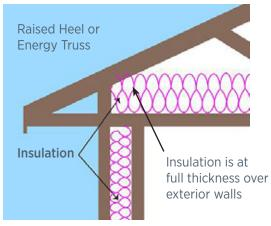
Insight Homes are built with raised-heel energy trusses, which can accommodate a full 14 inches of insulation over the whole ceiling deck including the top plate, eliminating cold spots along the tops of outside walls.
