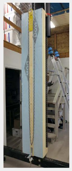
Full-scale assemblies were used to limit variations in installation from affecting the test results. Over the course of the testing, several test iterations were completed that varied insulation type and fastener spacing.
