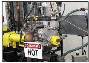
Vehicle components are operated real-time in an emulated vehicle context
